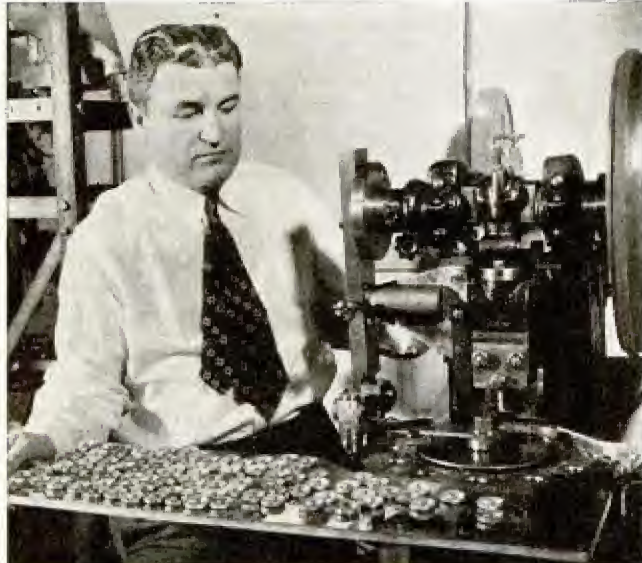
Machine making caps leakproof by stamping two concentric circles which form a new seat of contact with bottle top
